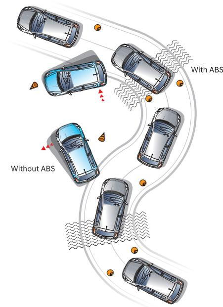
Anti-lock Braking System (ABS)
